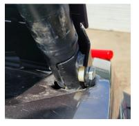
Next you will put the fender brackets on if you want the fold down option. On the front fender by the headlights there are two bolts. You will remove those and place the bracket on the fender and bolt in place with stock bolts. Leave loose for adjustment. Lay the window down and line up the holes with the pin. Now tighten your bolts and it should hold everything in the line up position. You're now ready to ride.
